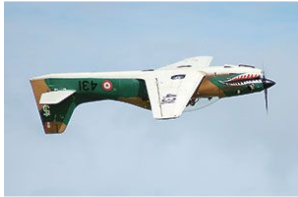
Modern aerobatic aircraft have flat, square wing tips to help them stall more easily!
