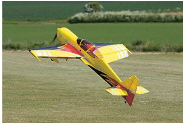
Power, light weight and large control surfaces are everything when flying in high alpha.
