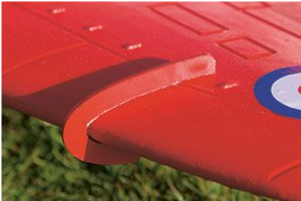
Wing fences stop air spilling out along the wing, which helps to improve the stall characteristics.
