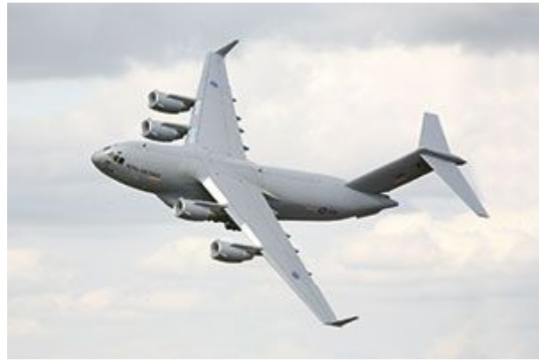
If an aircraft is in a banked turn of, say, 60°, the stalling speed can increase by as much as 40%.
