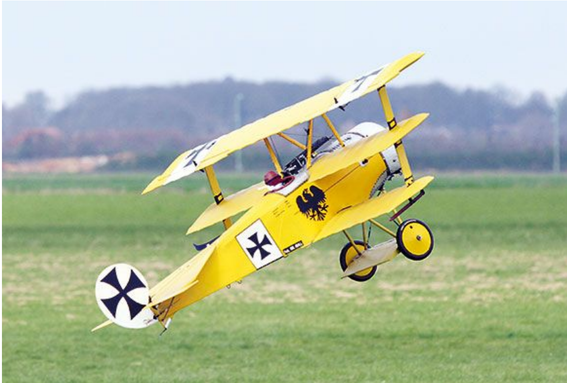
Short-coupled W.W.I types can be tricky on the ground and are one example where long take-off runs are best avoided. Fortunately, their light wing loadings allow flying speed to be achieved quite quickly, just like the full-size!
